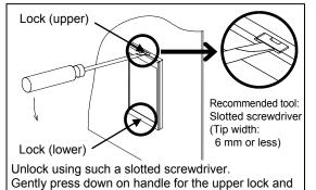
Apply pressure very carefully when removing internal assembly to avoid damage to the frame.
